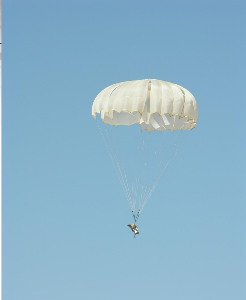
Extended Skirt Maltese Cross – late stage inflation
