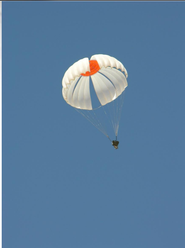
Slotted "Maltese Cross" Aeroconical Parachute
