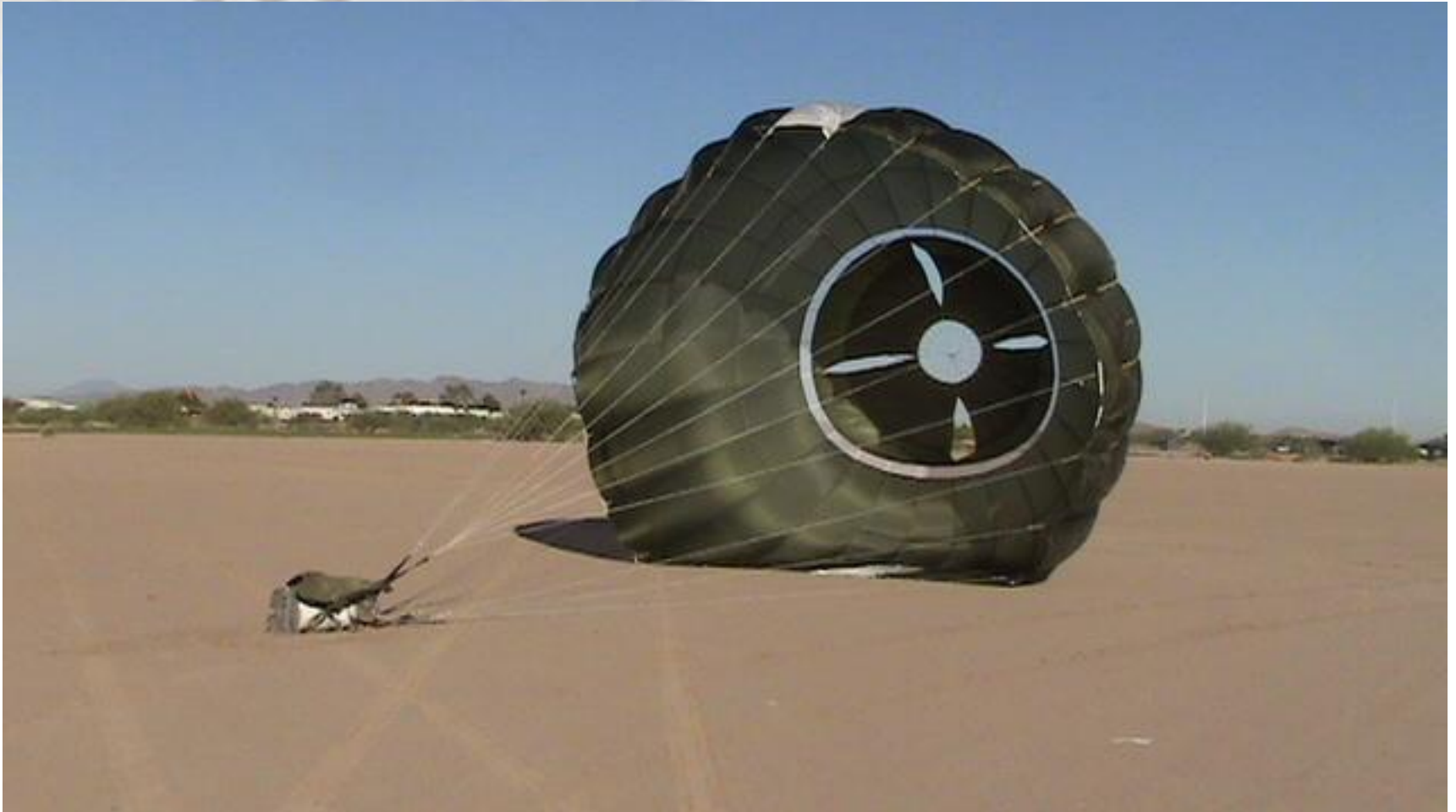
Standard Profile Type 6000 with Inflation Control Band and Crown Slots
