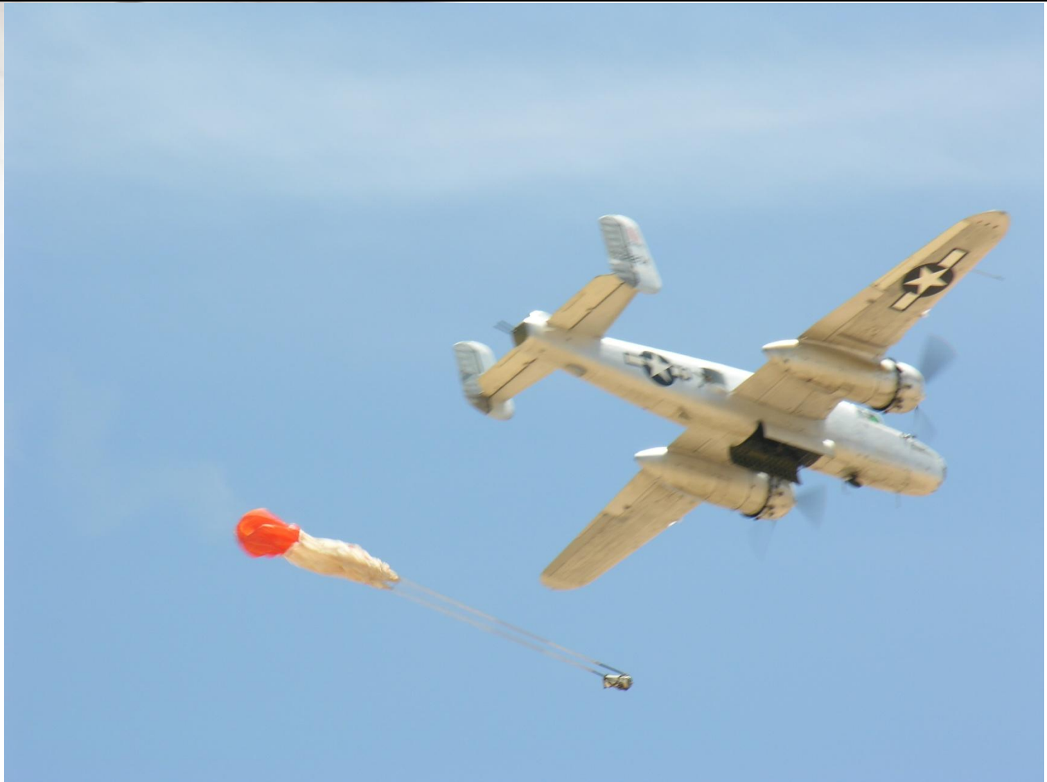
Early Phase Parachute Deployment
