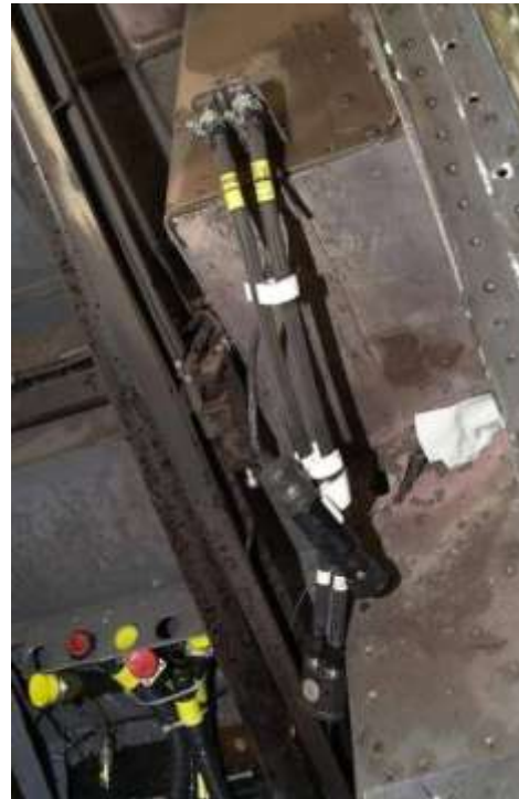
PCU hose assembly post test
