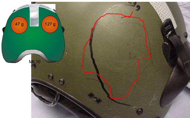
Figure 2: Photograph showing damage area detected using ultrasonic and vibration NDE techniques.
