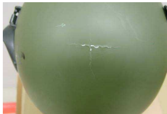
Figure 8: Impact damage on the top of a Mk10 helmet after an impact from 0.5m.
