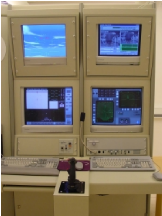
Fig. 6. Instructor Operator Station
