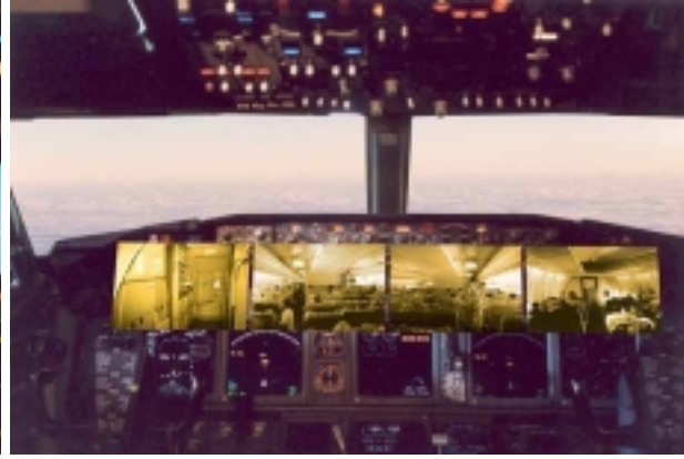
Fig 14. Line-display in cockpit showing virtual images from cabin
