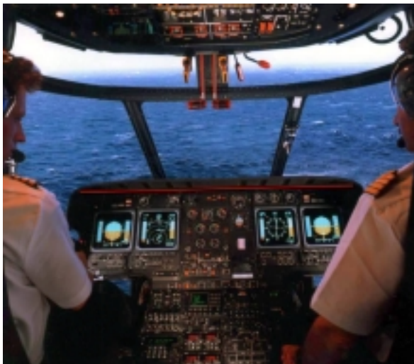
Fig. 11 Line-display helicopter installation.
