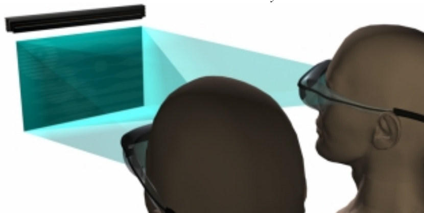
Fig.5 Linus is a "virtual panel display". As for the physical panel display, the image remains fixed in the room when the head moves
