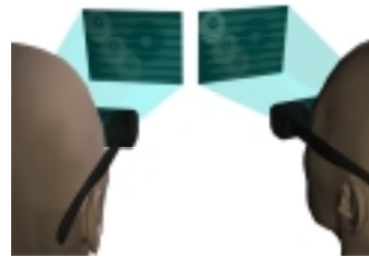
Fig.4 Micro Display Images follow the head movements and may cause motion sickness
