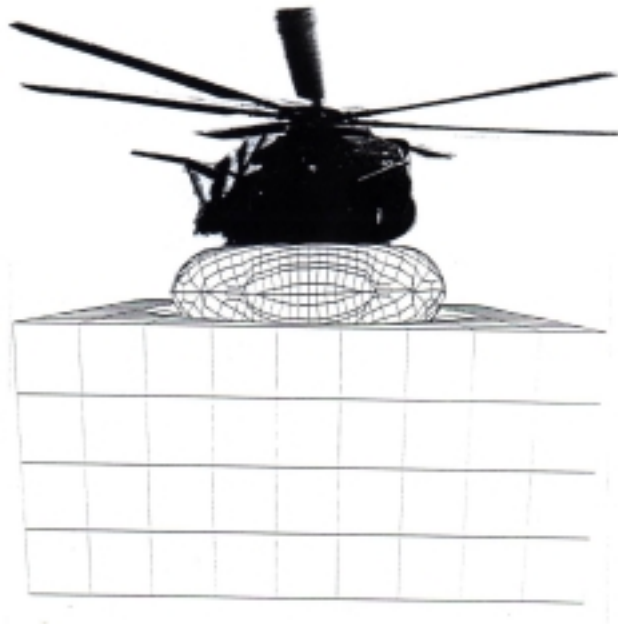
Figure 11. Conceptual scenario of helicopter falling into water protected by an airbag
