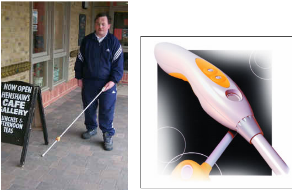
Figure 5: The UltraCane by Sound Foresight Ltd is a tactile navigation system for the blind.
