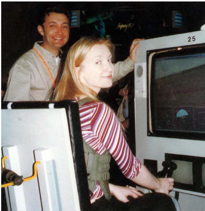
Figure 1: Tactile Situation Awareness System (TSAS), NAMRL, is a vest lined with vibrating 'tactors', which provides navigation and orientation cues to the pilot, seen here worn by Heidi Castle.
