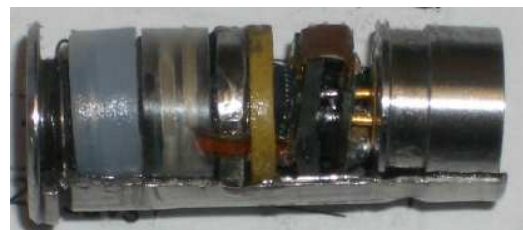
Photo 5: Pacific Scientific Delay Cartridge Sectioned View
