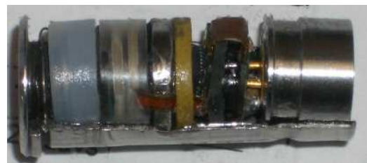
Photo 5: Pacific Scientific Delay Cartridge Sectioned View
