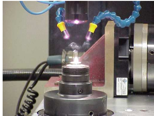
Photo 6: Example of Cartridge Laser Welding
