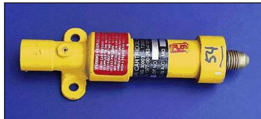
Photo 2: MC50 Cartridge Actuated Initiator
