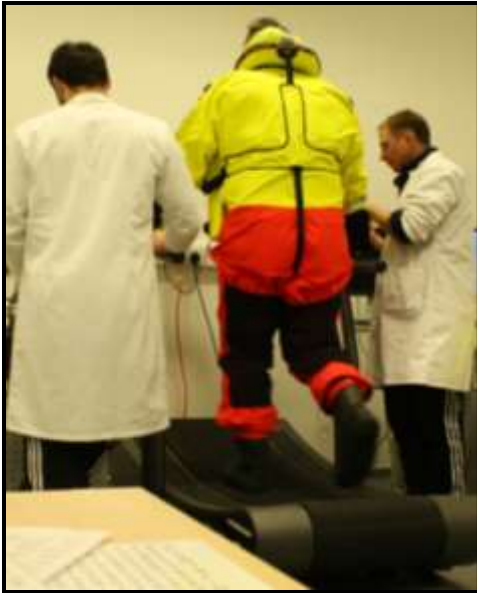
A pre-flight walk-out exercise of 5 km/hour for 5 minutes walk on a non powered tread mill
