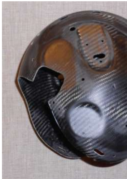
Rear of JSF helmet shell showing removal of knob of the standard ALPHA ratcheting system
